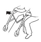
**BACK WHEELS** Large rear wheels should be inspected at least once a month to ensure proper tightness. If wheel wobbles or is loose, release lock nut and tighten axle bolt slightly. Test for proper tightness by leaning chair to one side and spinning adjusted wheel.
