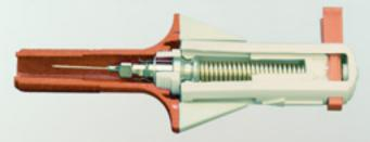
B. After the red safety latch is removed and the B.I.G. device is triggered under direct pressure, the spring is released and drives the needle.
