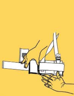
1 Remove and unfold the outer shaft assembly.
