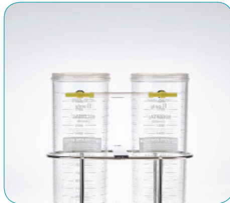
2. Connect canister "T"s with vacuum tubing.
