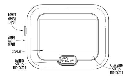
2. Next, locate the handle and plug the attached cable into the video cable input on the side of the display unit by aligning the white hash mark on the handle cable with the white hash mark on the side of the display. The plug and receptacle are shaped to fit only one way. <u>DO NOT</u> force or twist the plug into place.
