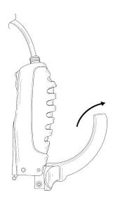
5. Finally, attach a new CoPilot VL®+ disposable sheath to the video blade. With the video blade open, slide the disposable sheath over the end of the video blade until it snaps into place.
