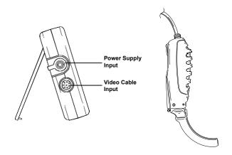
**4.** To turn the device on, simply open the video blade. The LEDs will illuminate and an image will appear on the display.
