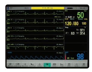
The **Omni (K)**<sup> $\mathsf{M}$ </sup> offers a 3, 5, and 12 lead ECG platform. Arrhythmia detection and ST are also standard and measurable on all lead sets.
