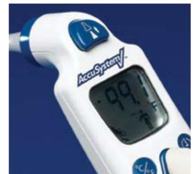
To recall the last temperature, press and release the scan button before loading another probe cover. Loading a new probe cover will erase the last temperature taken from memory.
