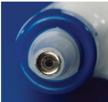
Inspect the membrane on the end of the probe cover. If a hole or tear is visible, discard and attach new probe cover.
