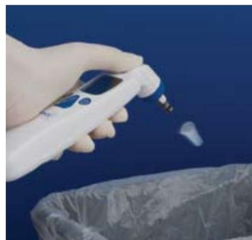
Dispose of the probe cover into a waste receptacle by pressing the eject button.
