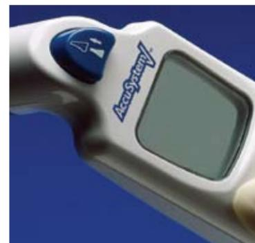
LCD display will go into "sleep" mode after 10 seconds of inactivity.
