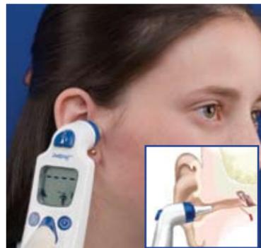
Insert the tapered probe tip. Align the probe at the entrance of the patient's ear canal.
