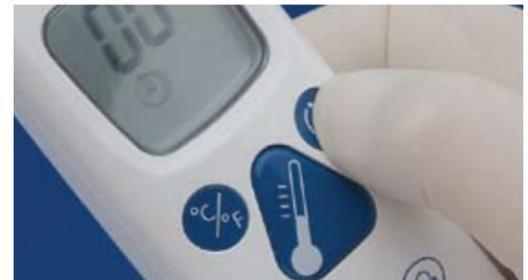
Press and release the (clock icon) once to begin (beeps will be heard at 15 second intervals) and it will automatically shut off at 60. If finished with function prior to complete 60 seconds, press and release (clock icon) a second time to deactivate function.
