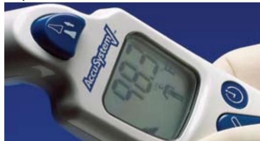
To change the temperature display press and hold the C/F° button for 2 seconds when the LCD screen is active.
