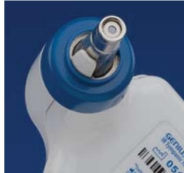
Inspect the probe lens. It should be shiny and free of cracks or debris without a probe cover attached. (Clean lens with a dry lint-free swab or lens wipe if needed.)
