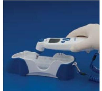
Attach probe cover by aligning the silver tip with a probe cover and push straight down until you hear a snap.
